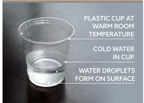
Fill a glass with cold water. After a few seconds you'll notice small droplets on the outside of the glass up to the level of the water. This is condensation, formed as warm air cools on the glass. The same principal applies to your home.
